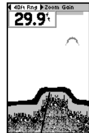
Structure is soft, probably a mud pile
