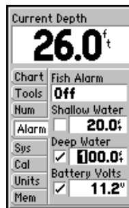
Deep Water Alarm
